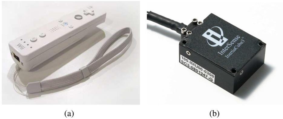
**Figure 2.4:** Inertial device examples. (a) Nintendo WiiMote incorporates inertial accelerometers. (b) InertiaCube 3, a hybrid inertial device that includes accelerometers, gyroscopes and a magnetometer.
