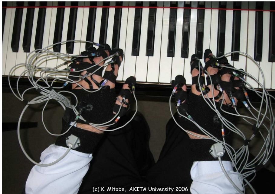
**Figure 2.10:** Hand motion capture system employing Polhemus sensors attached to a user's fingers. (Reprinted with permission from Kazutaka Mitobe - Akita University)
