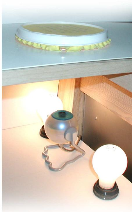
**Figure 2.11:** Camera viewing the underside of a malleable surface. (Reprinted with permission from Florian Vogt - The University of British Columbia)
