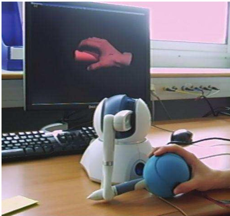
**Figure 2.15:** Phantom haptic device with five pressure sensors attached to grip allowing virtual clay sculpting. (Reprinted with permission from Adeline Pihuit - University of Grenoble and INRIA)
