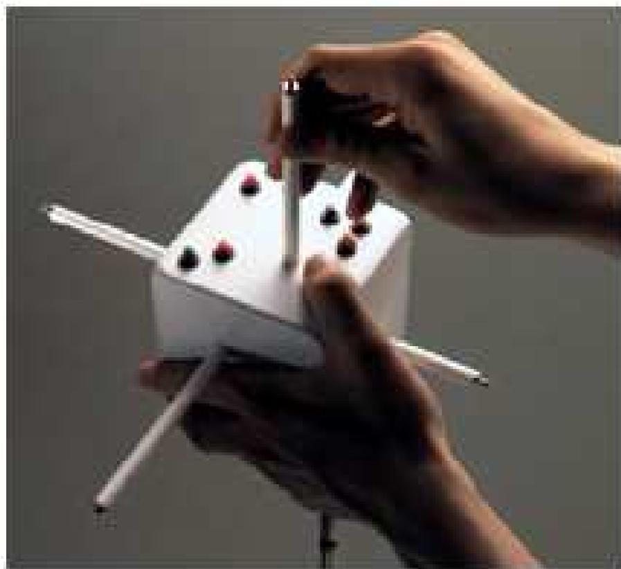
**Figure 2.14:** The Cubic Mouse a 12 DOF input device. (Reprinted with permission from Bernd Fröhlich)
