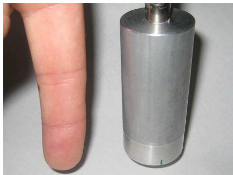
**Figure 6.6:** Mechanical finger modified to a 36mm diameter
