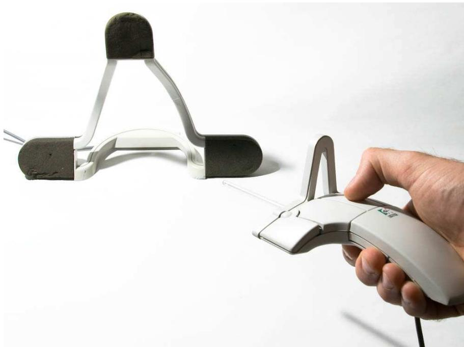
**Figure 2.8:** Logitech 6 DOF ultrasonic pointing device.
